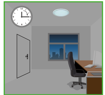
Light switches off automatically after the dimming time elapsed.
